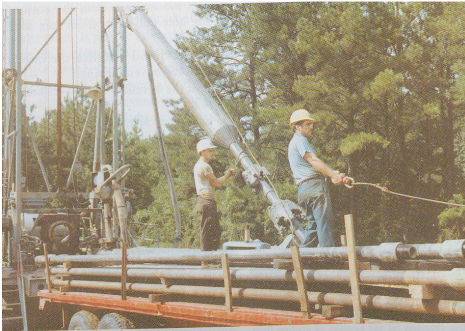
Figure 10.17. Heavy collars added to the drill string above the bit help keep the borehole straight.
