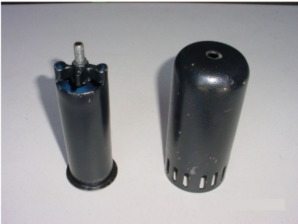
FIGURE 2-35 Bubble cap components.
