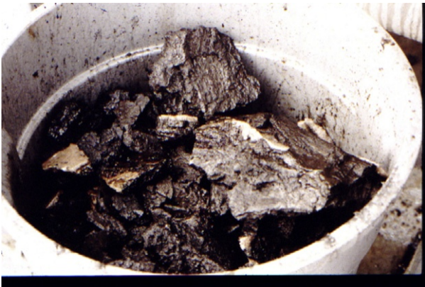
FIGURE 3-15 Heavy fractions of tarry hydrocarbons collected from bottom of reboiler.
