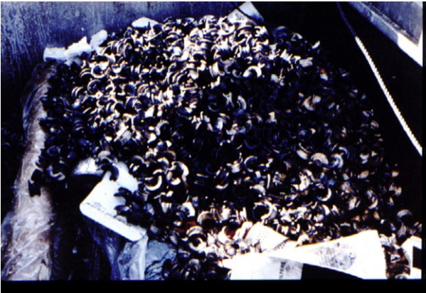
FIGURE 3-24 Ceramic saddles coated with hydrocarbon tar.
