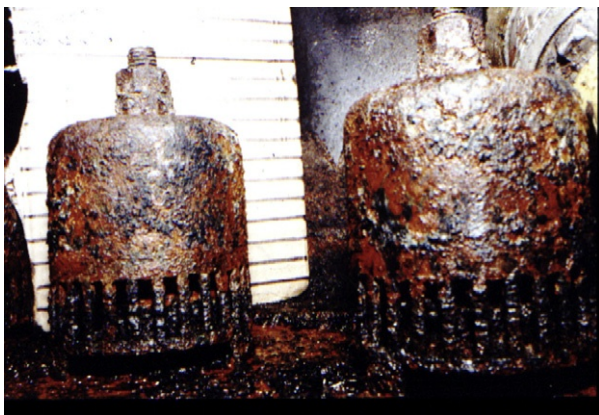
FIGURE 3-1 Oxidation corrosion of bubble cap tray.
