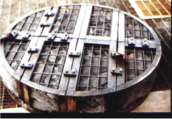
FIGURE 3-19 Replacement mist extractor. (Courtesy of Gly-Tech)
