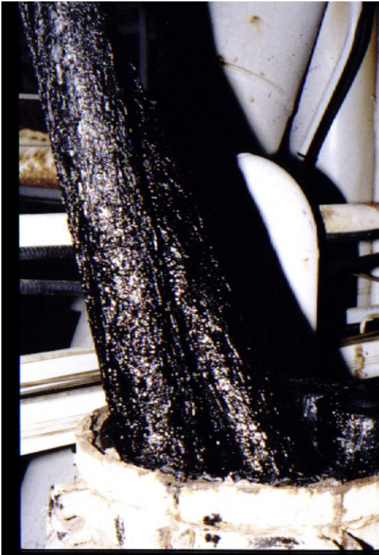
FIGURE 3-10 Sludge captured on glycol microfiber filters.
