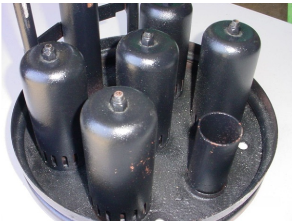
FIGURE 2-36 Bubble cap tray outside the contactor tower.
