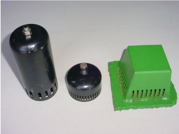
FIGURE 2-34 Common bubble cap configurations.
