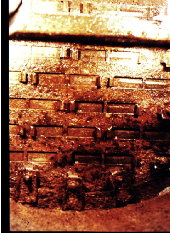
FIGURE 3-2 Sweet corrosion of valve tray.
