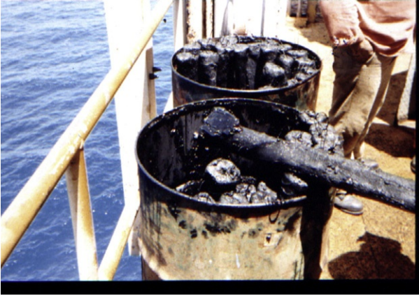
FIGURE 3-33 Decomposed glycol captured in the microfiber filters.
