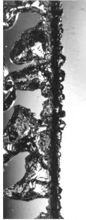
3.75 cm length of 0.164 cm diam. wire in benzene at earth-normal gravity. q=0.35 \times 10^6 \text{ W/m}^2
