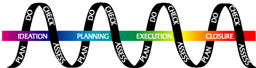
Figure 2.1-3 TCM Applies the PDCA Concept Throughout the Project or Asset Life Cycle
