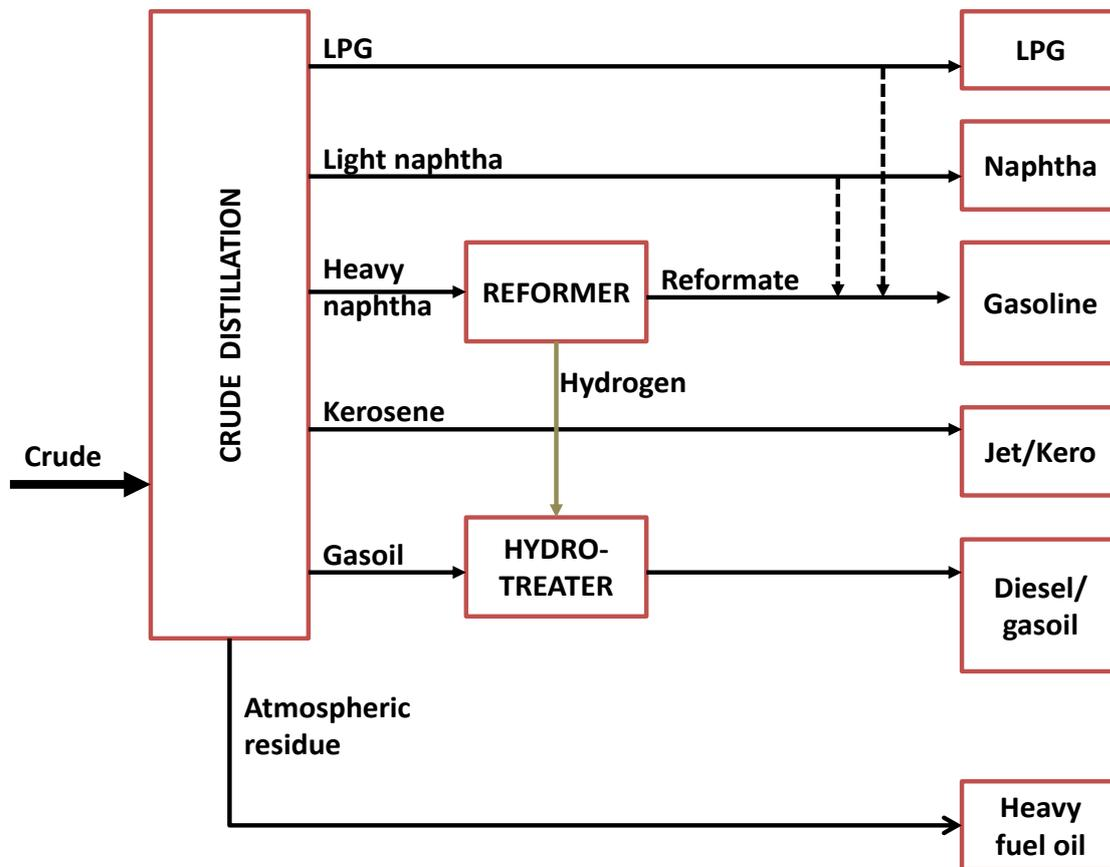
Figure 2.4 A Hydroskimming Refinery (Speight, 2011)
