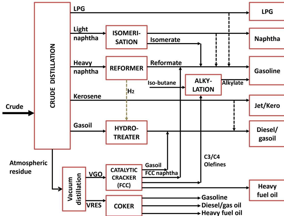
Figure 2.6 A Coking Refinery (Speight, 2011)
