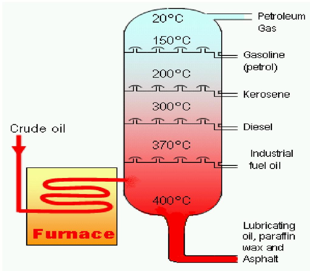
Figure 2.2 Simple Fractional Distillation (Pighadshy, 2008)
