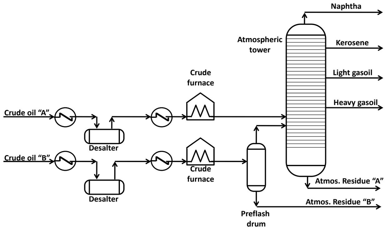
Figure 5.5 Most effective refinery scheme (Dual Drum Scheme: Hori, 2000)
