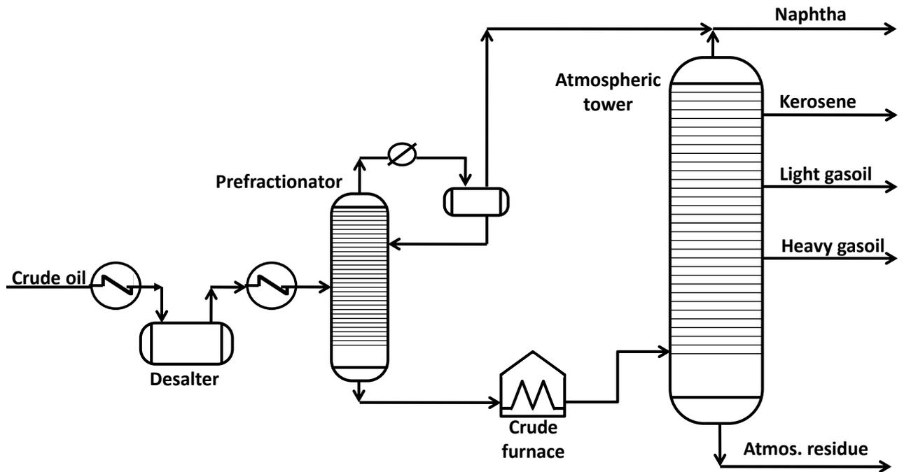
**Figure 5.2 Prefractionator Scheme (Hori, 2000)**
