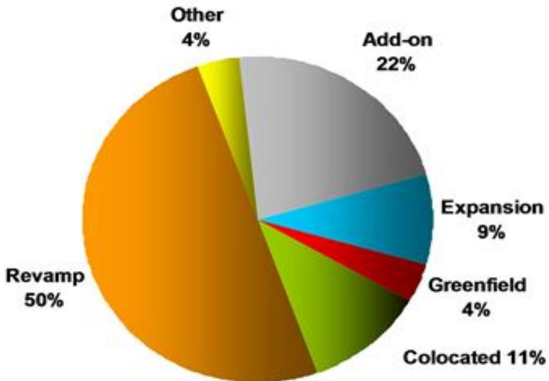
Figure 2.7 Refinery Project Type (Independent Project Analysis, 2009)
