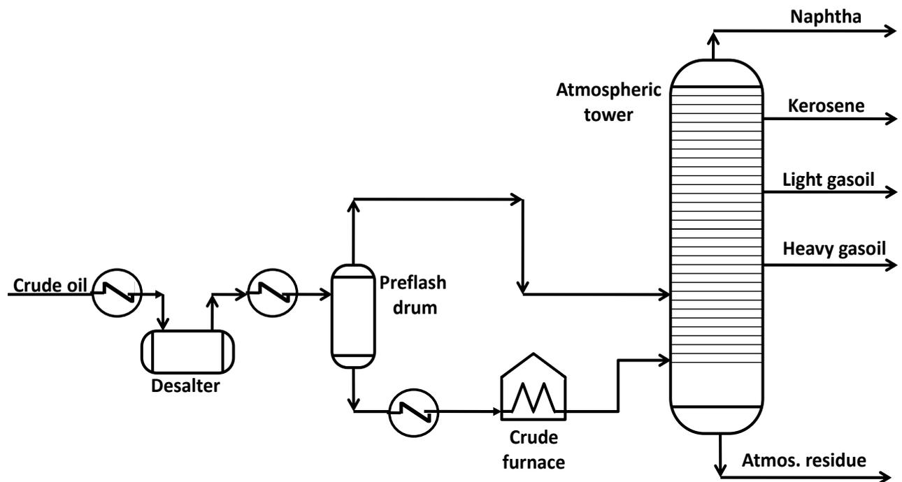
Figure 5.1 Preflash Drum Scheme (Hori, 2000)
