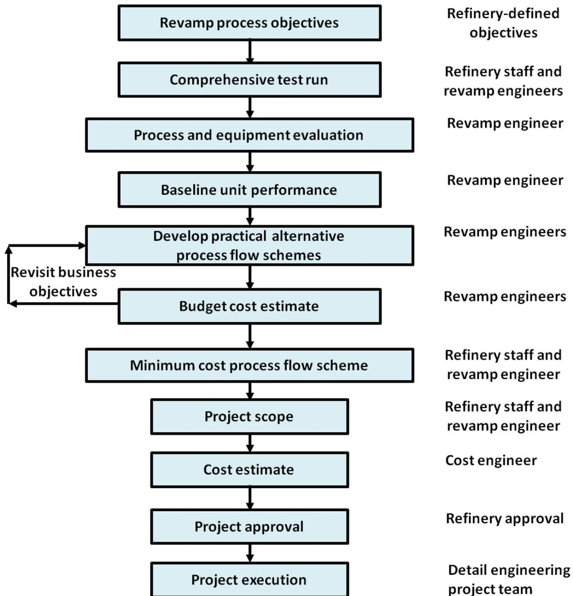
Figure 4.29 Revamp execution - logic-based approach (Golden, 2003)
