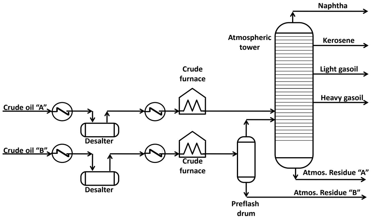
Figure 5.3 Dual Drum Scheme (Hori, 2000)
